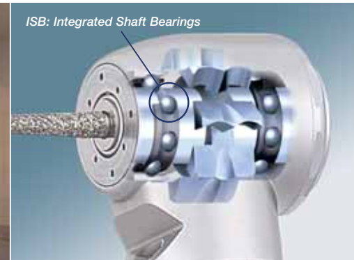
Integrated Shaft Bearings (ISB), the shaft itself forms an inner race for holding outer race, ensures vibration-free, accurate and stable cutting.
