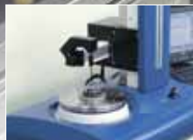
High-precision roundness measuring equipment: Core vibration is crucial to rotating equipment. Perfectly round rotating parts are necessary to achieve zero core vibration. Roundness is measured to an accuracy of 0.01 \mu\text{m} . (0.00001 mm)
