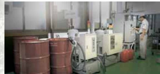
Precision filter achieved a recycling rate of 97% for cutting oil.
